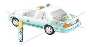
Ford offers the Fire Suppression System as a factory option. TFSS is an automotive industry first.
