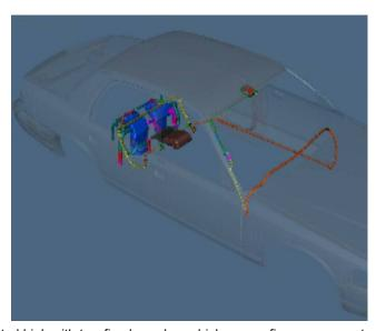
An additional manifold, mounted high with two fixed nozzles, which sprays fire suppressant material
